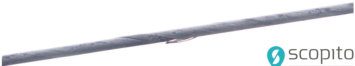
A damaged strand on a power line, captured by means of a drone. Image: Scopito.
