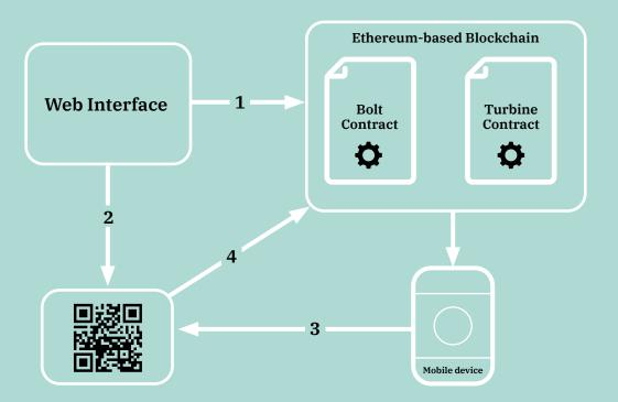
The registration phase consists of the following actions: 1. Supplier fills in bolt / turbine properties and adds the record into the smart contracts in the blockchain 2. QR Code to blockchain interface gets generated 3. Mobile device scans QR Code and follows the link 4. A call to the Smart Contract gets issued 5. Smart Contracts return the requested bolt / turbine record.
